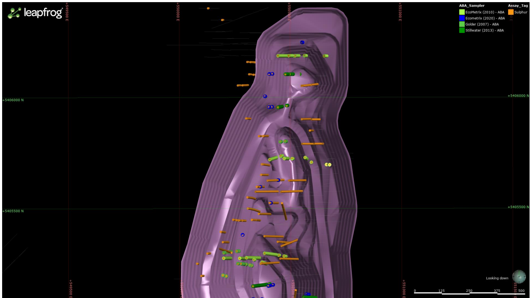
Appendix A-1: Northern extent of the pit with approximate sampling locations. 2020 samples are represented by blue cylinders. Previous samples analyzed for ABA and/or sulphur are represented by green and orange cylinders, respectively.
