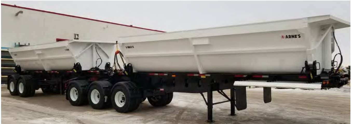
Figure 18.14: Example of Dual-trailer Side-dump Trailer with a Max 36-40 t Capacity
