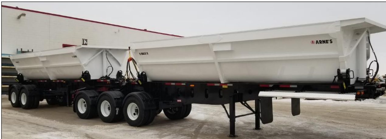
Figure 18-5: Example of Dual-Trailer Side-Dump Trailer with a Maximum 36 to 40 t Capacity
