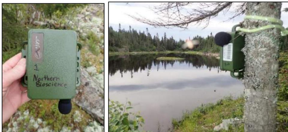
**Figure 3. Wildlife Acoustics SM Mini-Bat acoustic recorder (left) and lakeside deployment (right).**
