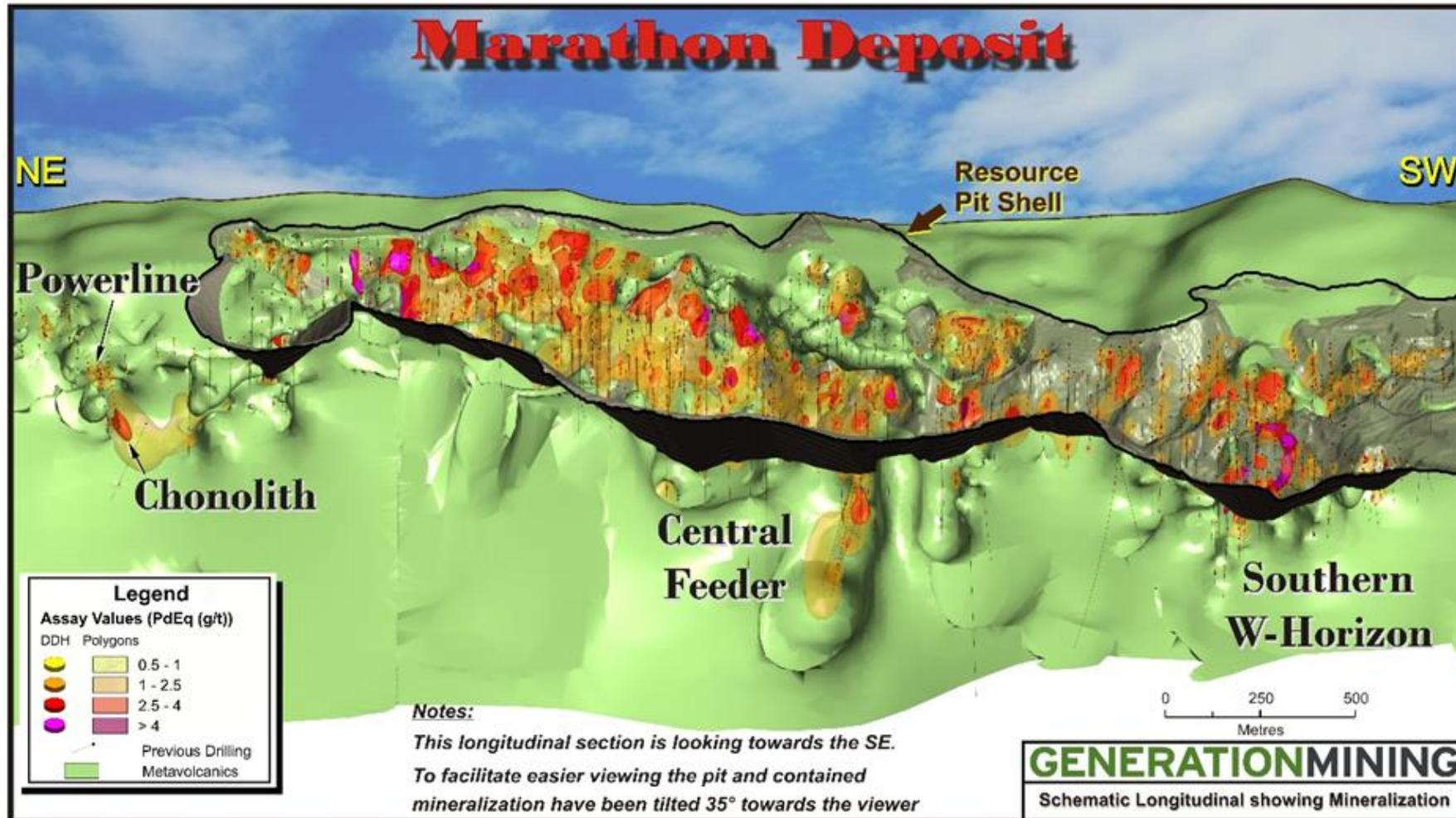
Highlights of 2021 Chonolith drilling: Hole 43, 16m @ 2.11 g/t PdEq; Hole 44, 80m @ 1.08 g/t PdEq; Hole 45, 46m @ 1.78 g/t PdEq and 37m @ 1.4 g/t PdEq
